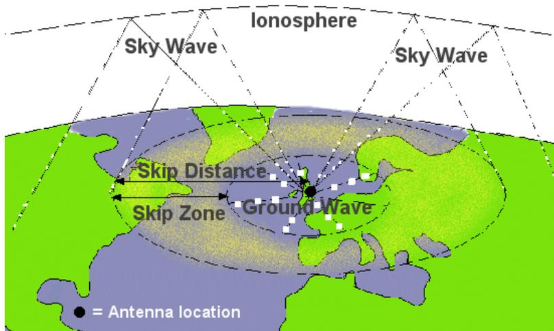
Our answer is not to increase power, try to set up VHF repeaters, or other drastic measures. The answer is simple, install an NVIS antenna, select the appropriate operating frequency, and reliable communications from 0 to 300 miles becomes very achievable.
