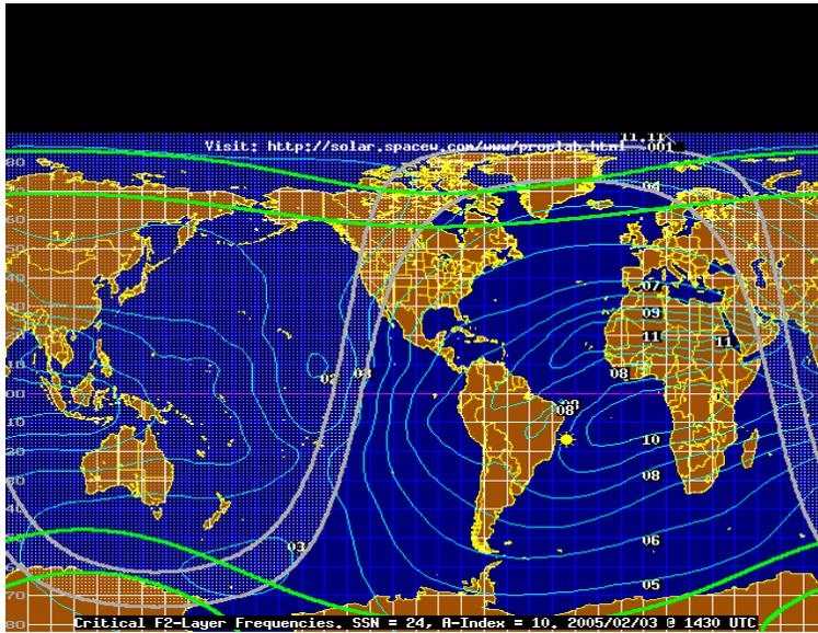
Fortunately, we can determine the best operating frequency from propagation information on the internet and some relatively simple calculations. A good place to find the F2 critical frequency is at <http://www.spacew.com/www/fof2.html>. An example is shown to the left.
