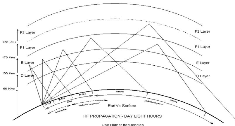
As the signals leave the antennas, they travel up and are refracted off the various ionosphere layers. The lower the signal's incident angle and the higher the layer of refraction, the farther away from the transmitter the signal returns to earth.
